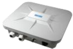
PLC AMI Medium- Voltage Head End
